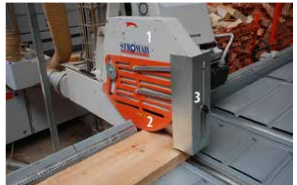
Covers on a crosscut saw. The fixed cover (1) always protects the upper part of the saw blade. The moving cover (2) follows the thickness of the wood as it runs over it. You set the adjustable cover (3) according to the thickness of the wood.
