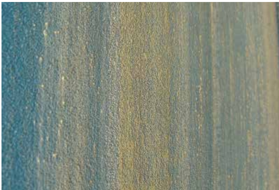
When the grit loses its sharp edges, heat builds up during machining, which causes sanding dust to adhere to the belt's surface and leave marks on the sanded surface. A worn belt can break and damage both the machine and the workpiece.
