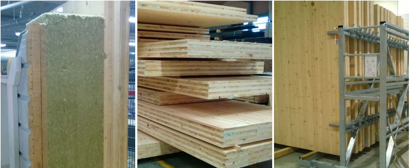
Cross-section through load-bearing CLT wall.
