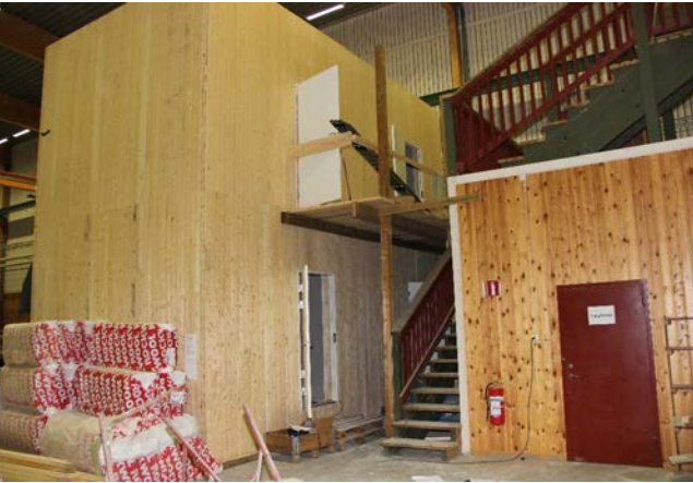
A test house designed for sound measurements, comprising 3 – 4 units.
