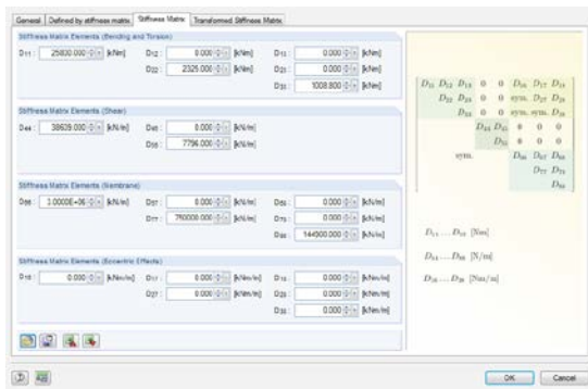
Figure 3.30 Example of what makes up a stiffness matrix for orthotropic surfaces.
