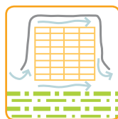
Ventilation under tarpaulin
