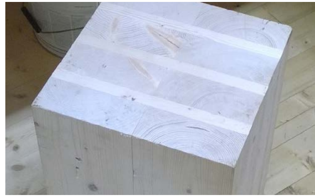
7-layer CLT block made from spruce.
