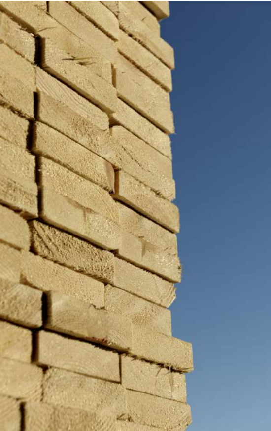
Boards to be used for CLT panels.
