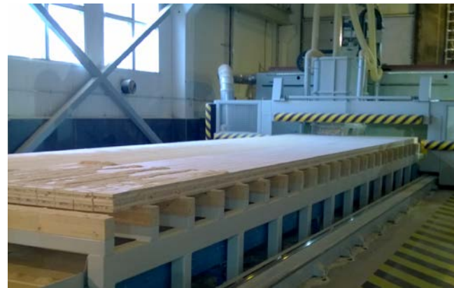
Finishing a CLT panel in a CNC machine, CNC = Computer Numerical Control.
