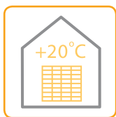
Stack CLT on stickers if it gets damp
